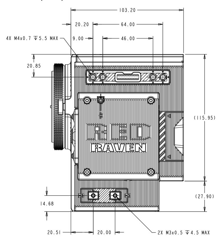
Figure: RAVEN Side View (Right)
