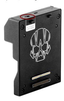
Figure: Auto Boot on Power Switch
