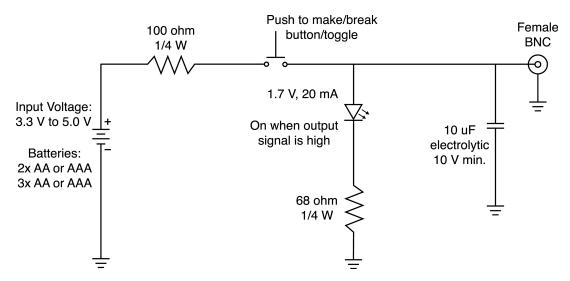
Figure: Trigger Button Circuit Diagram
