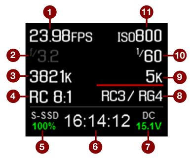
Figure: DSMC2 Sidekick OLED (Local Mode)
