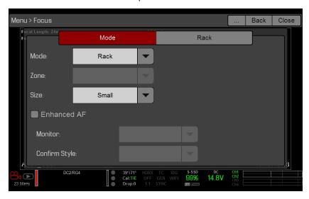
Figure: Set Up Rack Focus
